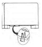
When removing the filters, treat the catches gently as they do not require much pressure and the lugs can be broken. To replace, locate carefully in the square apertures.
