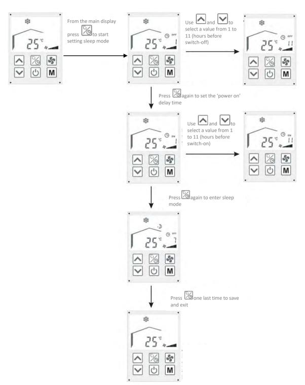
Note, if no button is pressed for 5 secs at any time during the setting process, whatever settings have been made will be saved and the display will return to the default display
