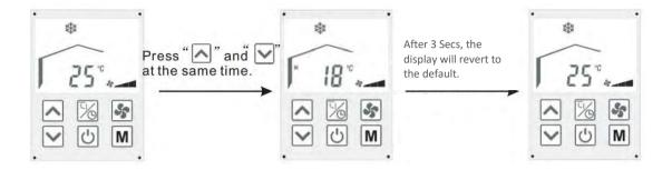
Turning the Air Vent on/off.
