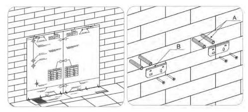
If you are going to use the Thermovec feet, they must be attached before installation as shown in the following two diagrams.
