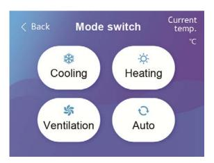
Cooling mode, to set the cooling temperature and fan speed, then to confirm. Heating mode, to set the heating temperature and fan speed, then to confirm. Ventilation mode, to set the fan speed, then to confirm.
