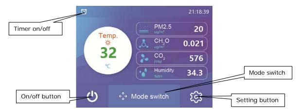
On/off button, to turn on or turn off the ventilator.
